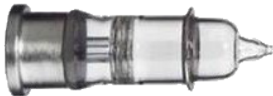
Fig. 1 DC discharge excitation lamp
